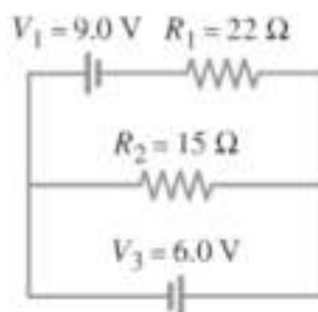
Determine the magnitude and direction of current through  $R_1$  and  $R_2$
