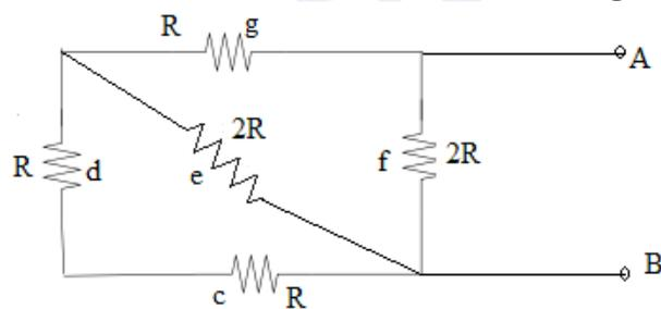
Resistors c and d are connected in series combination
